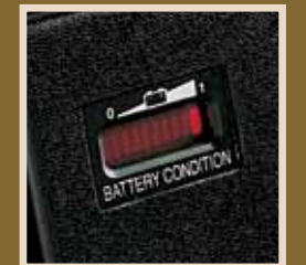
Battery Capacity Meter
